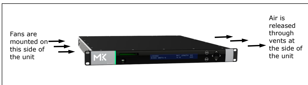
Figure 2.1 Air-flow through the Equipment
