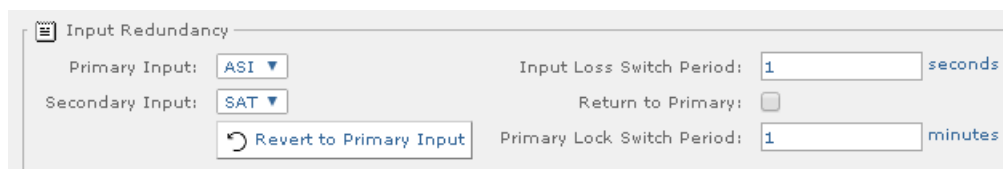
Figure 3-61 Configuration setting for Input Redundancy section
